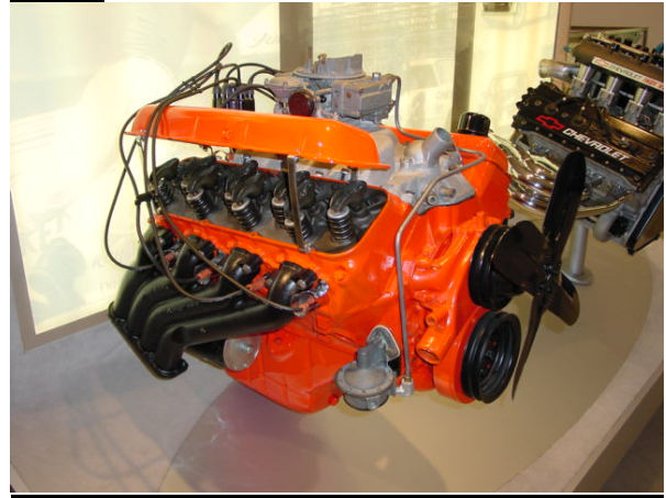
THE MARK II 427 MYSTERY ENGINE. FORE RUNNER OF THE MARK IV ENGINE
